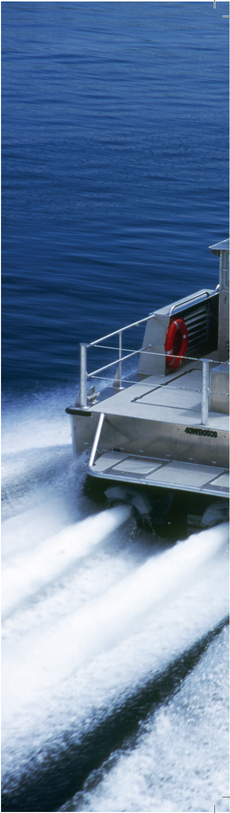
Right: Kvchak-built US Navy Maritime Prepositioning Force (MPF) high speed landing barge. Twin HamiltonJet HJ364 waterjets.
