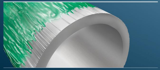
Metal tubes can have production-related longitudinal grooves or surface scratches. However, these faults can be compensated for by moistening the surfaces of the tube ends that are to be connected with LOKPREP fluid prior to assembly. Thanks to its capillary characteristic, it automatically covers the surfaces of the inserted tubes and flows into microscopic cavities and fills these out completely.
