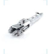
The hydraulic assembly tool enables the LOKRING connection of tubes with similar or different tube diameters. The production of the joining requires no special preparation of the tubes and can be carried out by unskilled workers. The tool is connected to the LOKRING hydraulic aggregate by a 2.8 m hydraulic hose. The sizes of the clamping and assembly jaws are dependent on the dimensions of the tubes that are to be joined.
