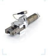
The hydraulic flaring tool is designed for the flaring of aluminium tubes for the production of LOKRING SINGLE RING tube joinings. It is connected to the LOKRING hydraulic aggregate by two 2.8 m hydraulic hoses. The forward and backward movement of the flaring insert is enabled by means of a double acting cylinder. The size of the clamping jaw and the flaring insert depends on the outside tube diameter.
