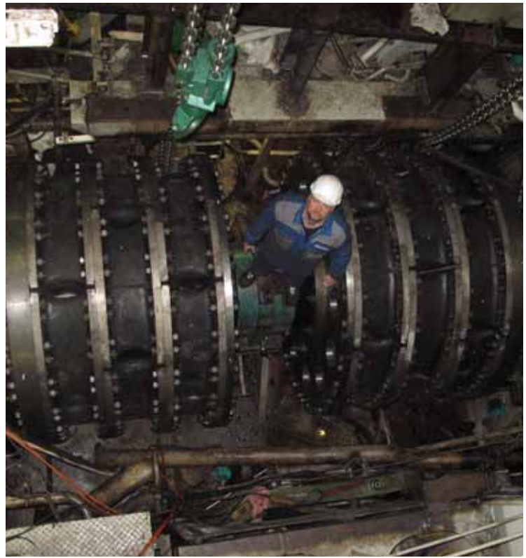
On the right: Finally it is done - two sets of two RATO S couplings are installed.
