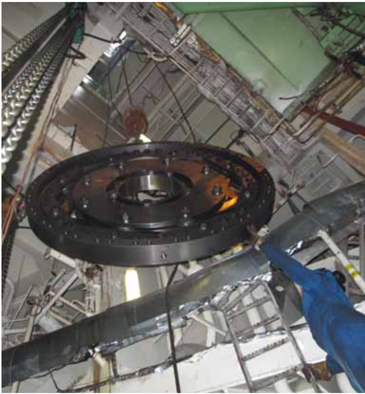
On the left: The link packages of the RATO S are lifted into the engine room by crane.
