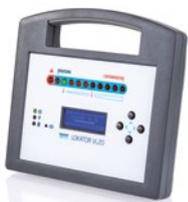
Mobile, industrial leak detector. The high flexibility of the LOKATOR VL20 allows for use with different refrigerants and for H<sub>2</sub> tracer gas with the same probe. The unit is the perfect tool for quick and accurate leak location whatever the gas to be detected.
