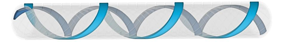
The composite coils of each layer are decoupled by gaps, the outer and inner layer are decoupled by high-performance elastomer material. This allows the coils to remain bending compliant which enables the entire shaft to be flexible in multiple directions. Additionally, the decoupling induces a virtually unidirectional force transmission through the composite coils which means high strains can be applied resulting in an excellent torsional elasticity.
