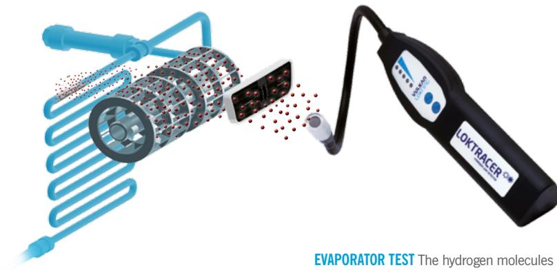
**EVAPORATOR TEST** The hydrogen molecules escape at the leak in the evaporator and get inside the passenger compartment through the ventilation slots.
