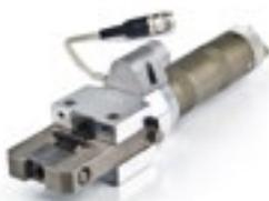
The hydraulic flaring tool is designed for the flaring of aluminium tubes for the production of LOKRING SINGLE RING tube joinings. It is connected to the LOKRING hydraulic aggregate by two 2.8 m hydraulic hoses. The forward and backward movement of the flaring insert is enabled by means of a double acting cylinder. The size of the clamping jaw and the flaring insert depends on the outside tube diameter.
